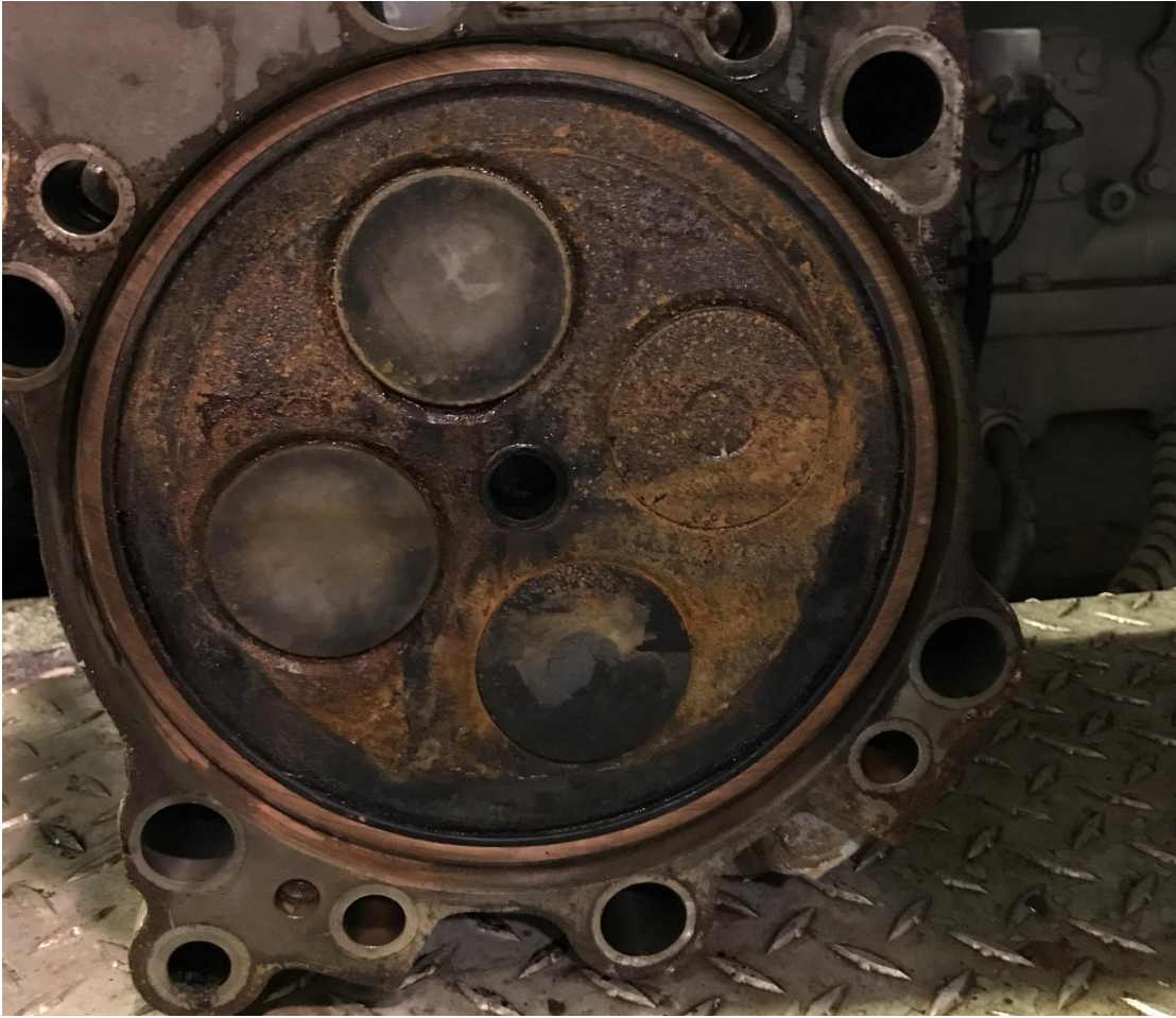
Figure 7 - Cylinder Head Condition with Intake and Exhaust Valves Installed
