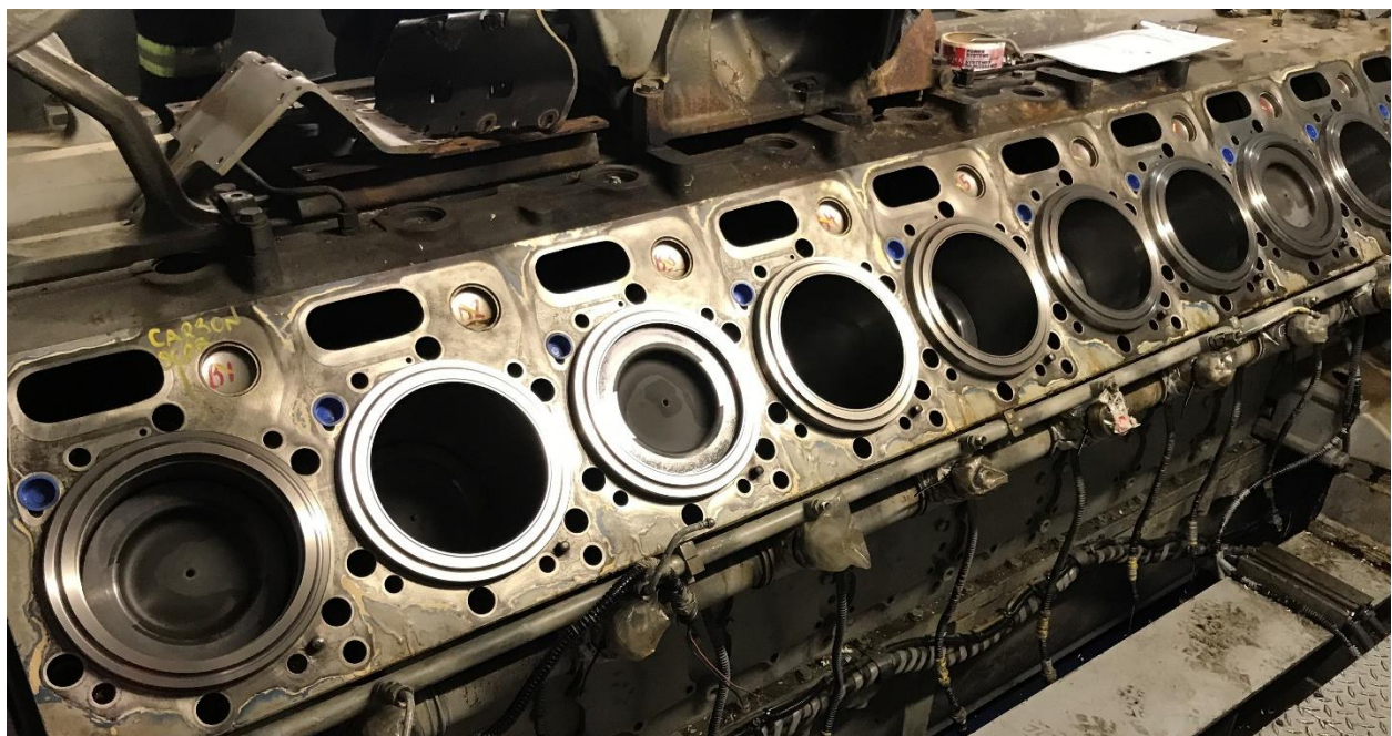
Figure 10 - New Cylinder Liners and OEM Refurbished Pistons
