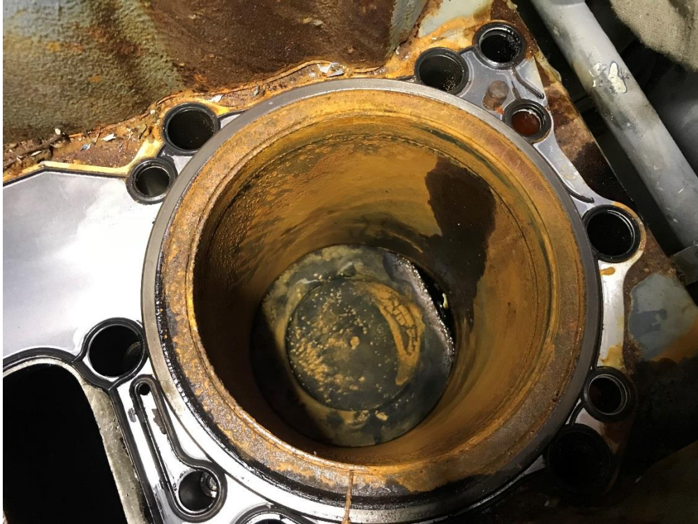
Figure 5 - Typical Cylinder Liner Condition. Corrosion Also Visible on Pistons
