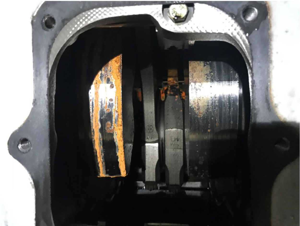
Figure 9 - Typical Surface Corrosion Observed on Crank Shaft.
