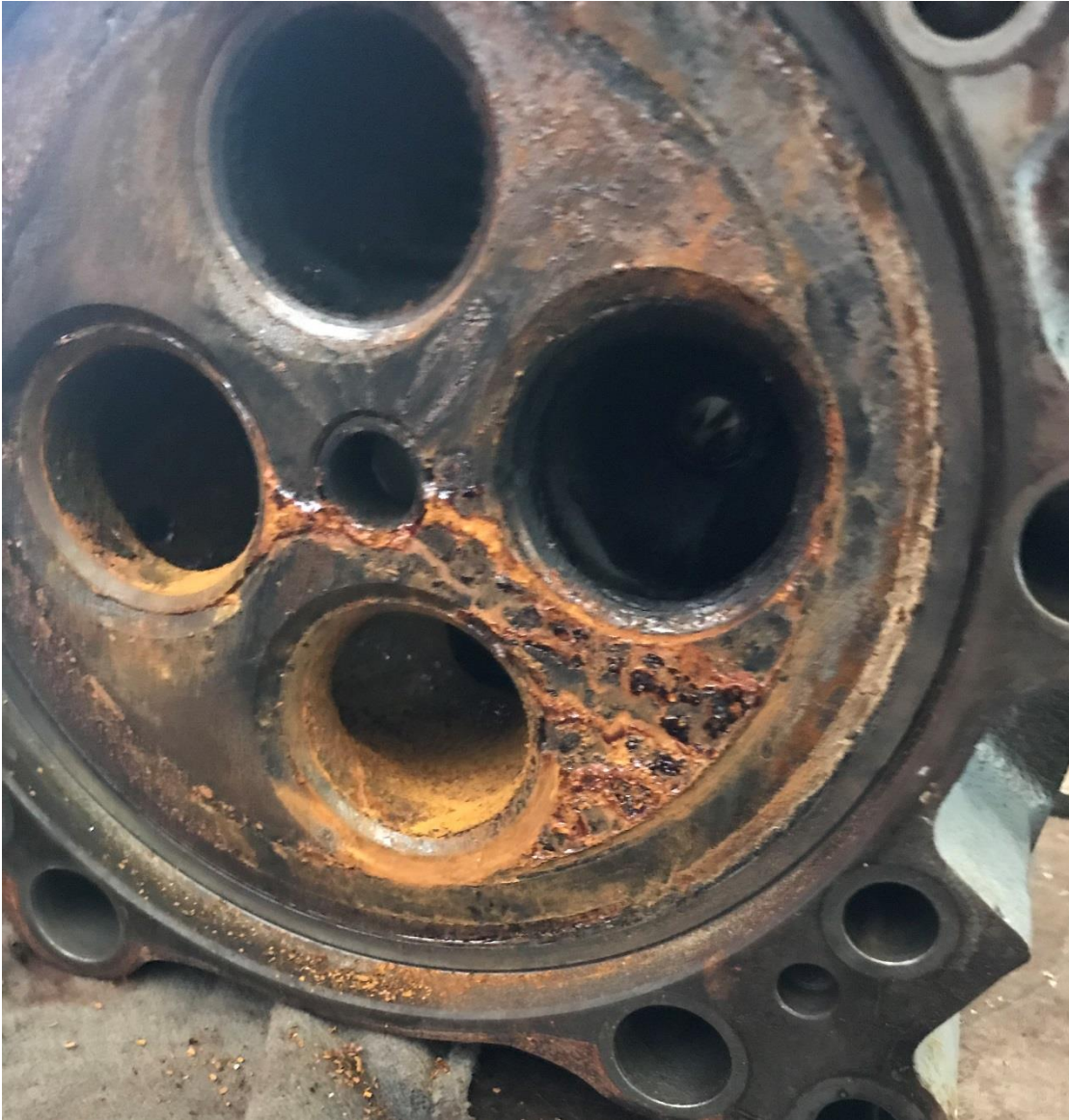
Figure 8 – Typical Cylinder Head Intake and Exhaust Valve Ports. Heavy Corrosion on Valve Seats
